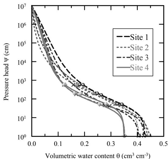
Figure 4 Water retention curves of the soil samples
