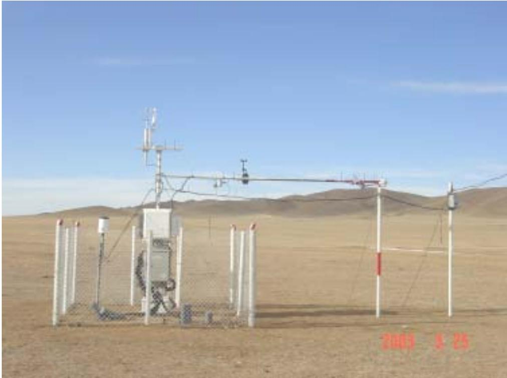
Fig. 13 A-1 Flux measurement system
