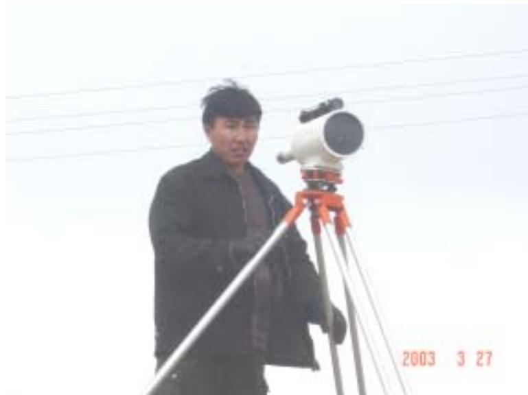
Fig. 15 The scintillometer receiver
